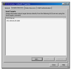
**10** If the connected ETERNUS DX Disk storage system uses multiple iSCSI ports, repeat the IP address addition process for each iSCSI port. (Repeat <a href="Step 7">Step 7</a> through <a href="Step 9">Step 9</a>.)
